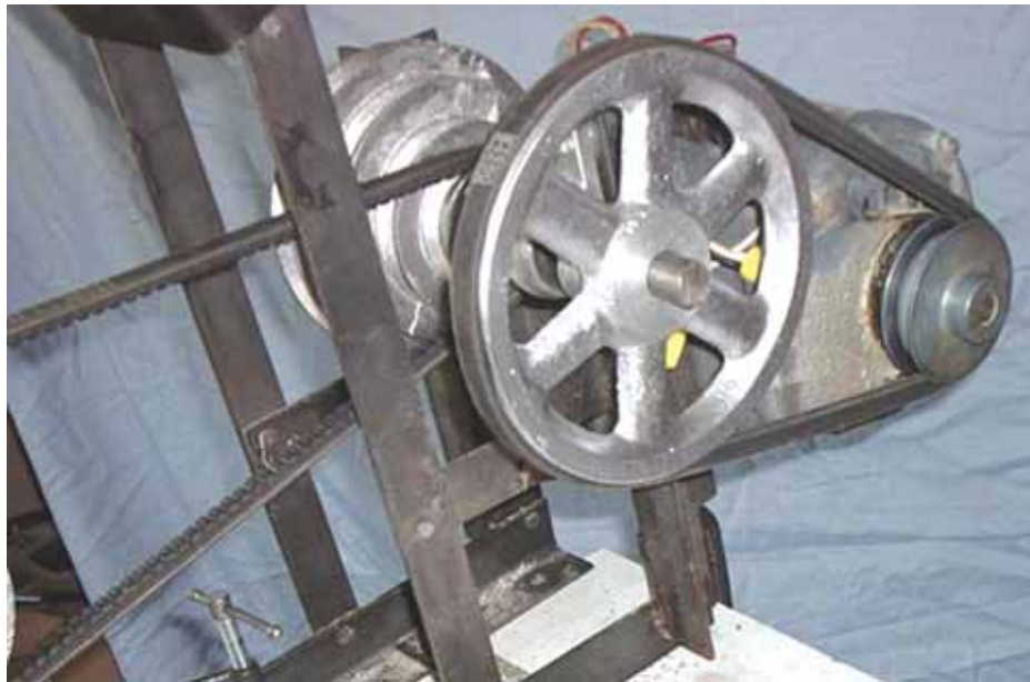
Compound belt drive
